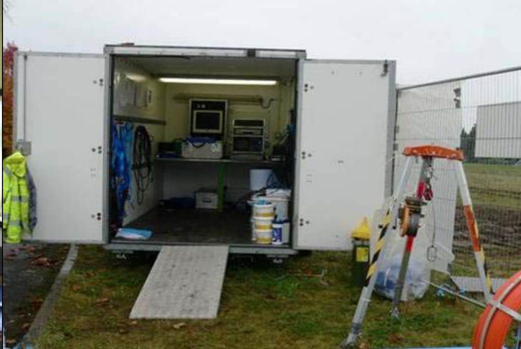
RSRL "Drover" Drain Probe System Used to Show Some Drains Can be Left In-Situ Clean
