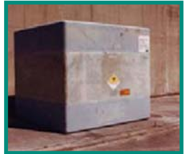
Typical ILW Container for Decommissioning Waste
